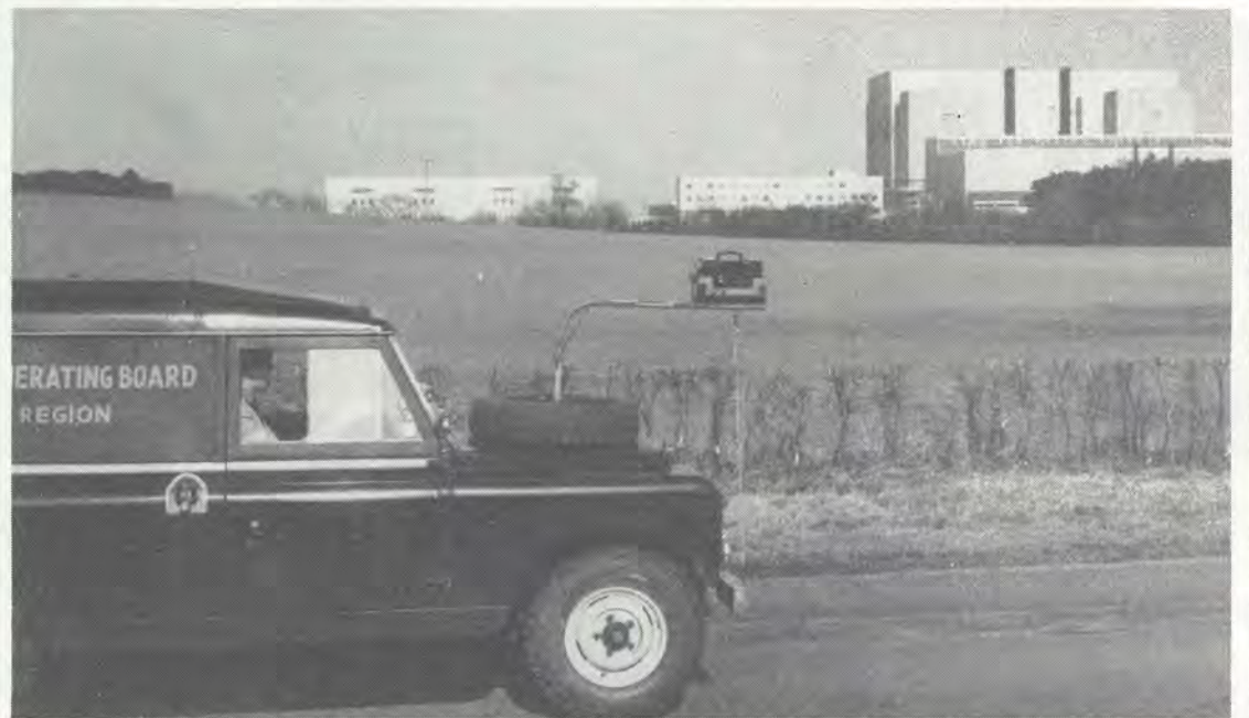
Safety measures at nuclear power stations include regular radiation monitoring. Here we see a gamma dose meter being used to check the grounds around the station
